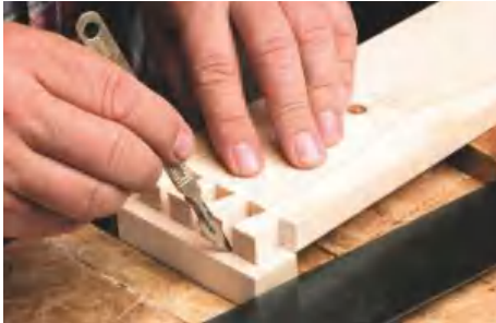
▲ Pic.10 Fine detailed work is demanding on the eyes so it needs plenty of light if you are going to make joints that fit well without gaps
